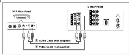
When connecting an external device, match the color of the connection terminal to the cable.
